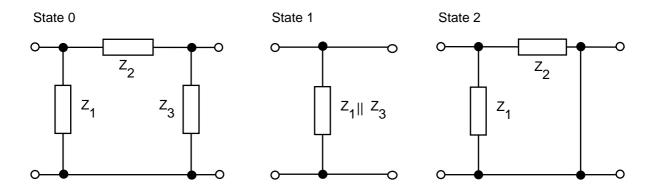
Figure 11: Switching states of the pi-network
