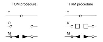
Figure 4: Manual calibration techniques.
