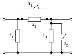
Figure 10: Switching unit realization.
