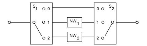
Figure 12: Realization of the switching network.
