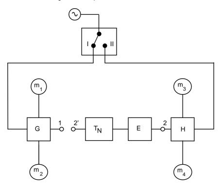
Figure 5: Configuration of the network analyzer.
