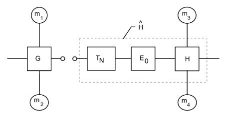
Figure 8: Initial state of the network analyzer
