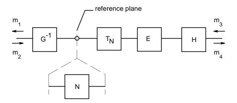
Figure 6: Realization of virtual calibration standards.
