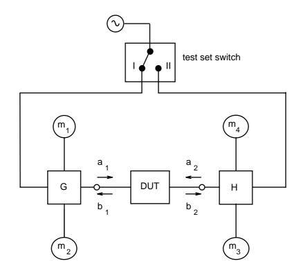
Figure 2: Block diagram of a vector network analyzer, e.g. ZVR
